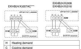
For heating-only applications, wire 17-C or 2-C is not to be installed.
