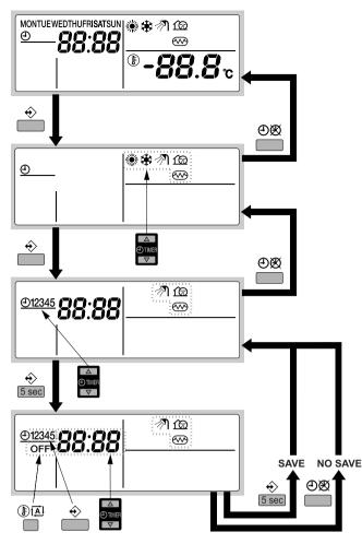
Programming sanitary heating, booster heater or silent mode is carried out as follows:
